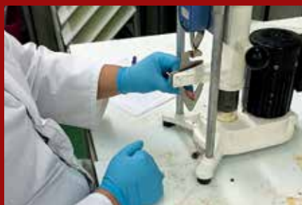
Meat cores are placed on the Warner Bratzler Shear Force and then a dull blade is drawn through the core and the amount of force required is registered.
