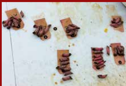
These are the cores taken from each cooked steak, parallel to the muscle fiber and devoid of fat pieces or connective tissue, ready for coring. Usually 5 or 6 are sheared to determine an average shear force.
